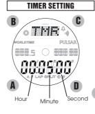
A Press to enter TIMER mode. Press and hold for 2 to 3 seconds to show TIMER SETTING display.
