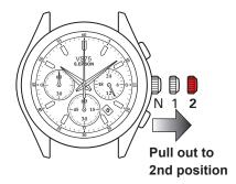
• Pull the crown out to the 2nd click position when the second hand is at the 12 o'clock position.
