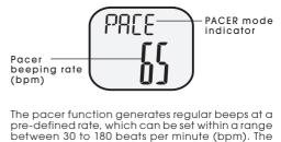
pacer and stopwatch can be activated at the same time. How to set the pacer beeping rate In the PACER mode, press Button D for 2 seconds to change the display to the PACER SETTING
