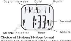
The time display format in either 12-hour indication or in 24-hour indication can be selected alternately by pressing Button B. Under the 12-hour indication format, AM/PM indicator appears on the display
