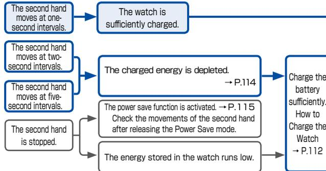
※ If the second hand does not move at one-second intervals even after fully charging the battery → "Charging the solar battery" in At Trouble on P.152
