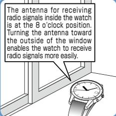
→ To enable the watch to easily receive a radio signal P.107
