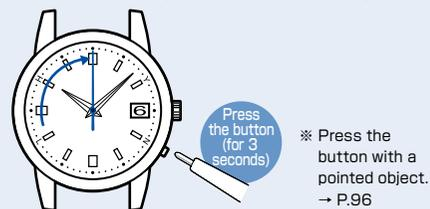
※ When the time difference is set for a region other than radio signal reception range, the second hand does not move to the zero second position (A radio signal cannot be received manually). Check the time difference set currently.
