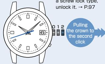
※ When the crown is a screw lock type, unlock it. → P.97
