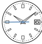
The second hand stops pointing at the 45-second position, and the hour and minute hands, and date also stop. The watch does not conduct automatic radio signal receiving. |
