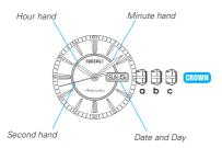
a) Normal position winding up the mainspring (manual operation)
