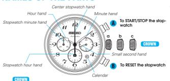
winding up the mainspring (manual operation) date setting a) Normal position
